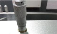
纵向“0”刻度对正刻度杆上的中标线，
